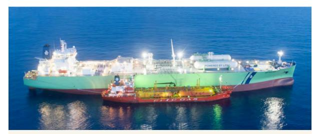
Our innovative use of established shipto-ship transfer (STS) practices for LPG bunker and coolant, pre- and post-drydock, has reduced turnaround time, increased commercial availability, minimised emissions, and allowed us stricter control over product origin compliance.
